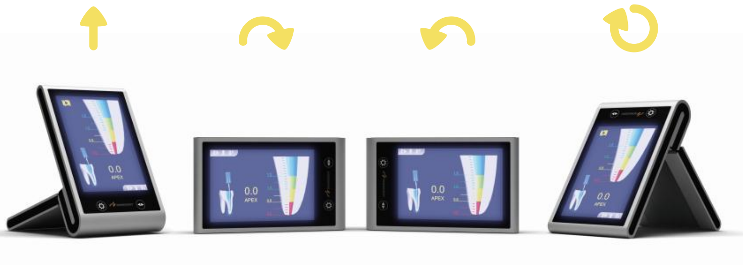
Equipped with high precision gyroscope, switch the display mode according to the state of display
